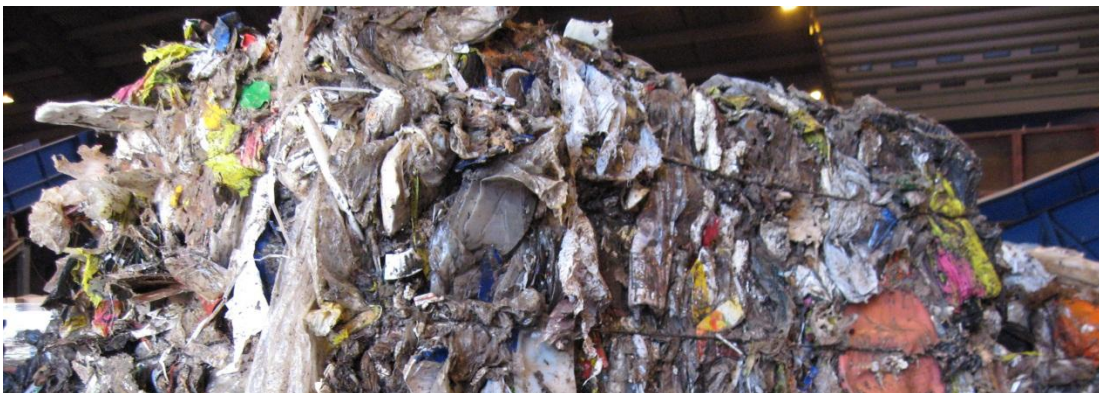
Figure 9 The baled mixed solid waste contains some plastic (the proportion of plastics measured as volume is high but not measured as mass)
