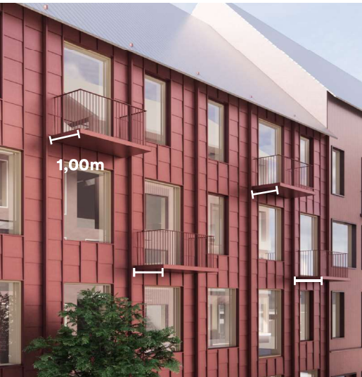
Max cantilevering 1 m. Light railing element
