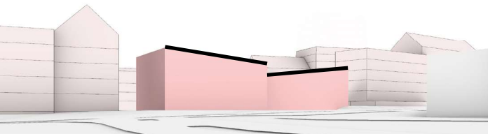
Angled roof profile inspired by the existing, massing relating to context while standing out.
