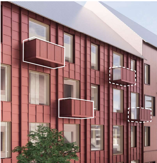
If closed Subdivisions and articulation, Either solid or glazed all-around, or solid front and glazed sides
