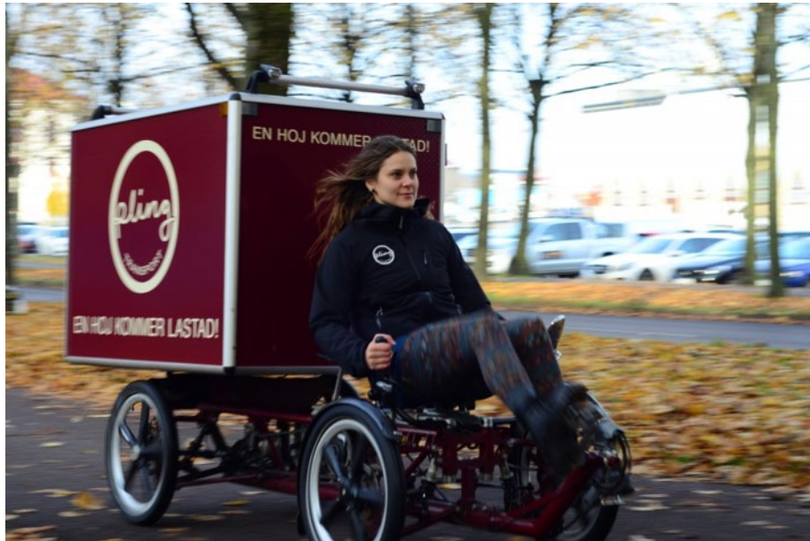
Image 3.5: A cycle courier with a cargo trailer capable of carrying up to two cubic metres per trip (Pling Transport, n.d.).
