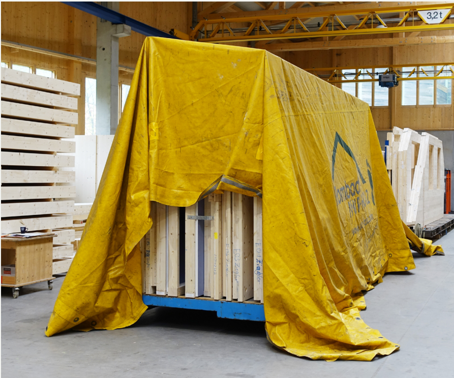
At the Rombach—NurHolz CLT factory in Southern Germany, the timber elements are wrapped for delivery in a reusable canvas.
