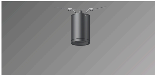
DAS140 TW LED IP66, Class 1, IK07, Marine-grade, die-cast aluminium alloy, SCE superior corrosion protection including PCS hardware, Silicone COC gasket, Safety glass lens, One cable entry, second cable entry for thorough wiring with cable connector optional, Integral EC electronic converter in thermally separated compartment, CAD-optimised optics for superior illumination and glare control, Factory installed LED circuit board, Tunable White Technology. The luminaire is factory-sealed and does not need to be opened during installation. Optional 2200 K version available. To be specified at time of ordering. Includes cable connector, for cable 2-12 mm, +/- 10° adjustable to compensate for sloping catenary systems.
